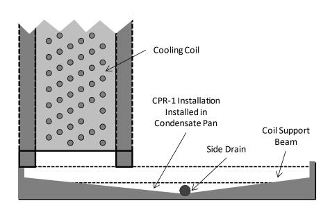
Side View of Drain Pan (Cross Section View of Coil)
