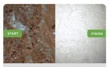
Probiotic foam from coil at the start (left) and finish (right) of the Tube Restoration Process.
